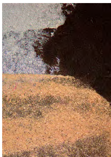
Fig. 91. Photomacrograph showing the metallic appearance and iridescent shimmer of lustrous pigments made by coating mica platelets with metal oxides or dyes. Field of view is approximately 7 x 12mm.
